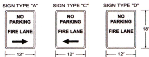
FIGURE D103.6 FIRE LANE SIGNS
